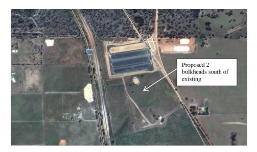
Each bulkhead will measure 250 metres by 35 metres with a 25,000 tonne capacity.
