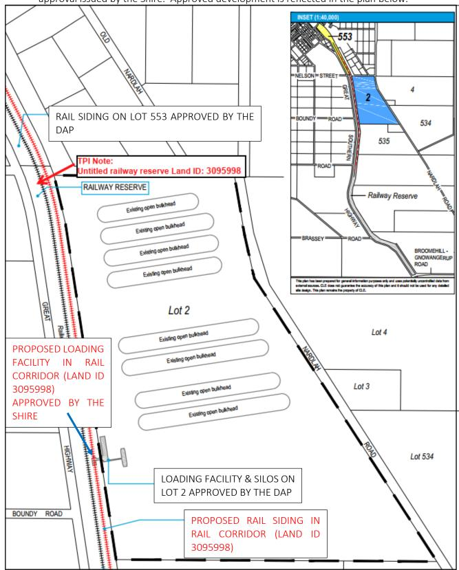
Note: The proposed railway siding extends further south than shown on this site plan extract. It has an approximate length of 1.6 kilometres.
